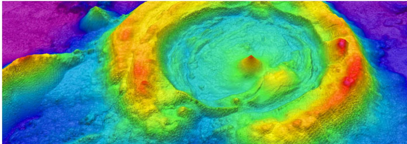
**LiDAR:** LiDAR (Light Detection and Ranging) uses laser pulses to measure the distance of an object to the source. The data points result in digital 3D maps for accurate design and engineering. LiDAR surveying crews use mobile (car or aerial vehicle) or static (tripod) equipment.
